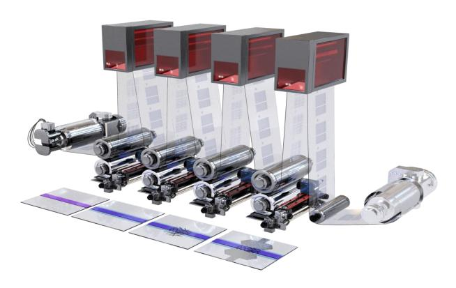
R2R in-line printing process for printing 4-bit processor via repeating rewinding and printing cycle 6 time to print active (3) to n-doping (8)
